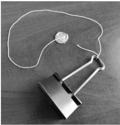
Pendulum Drop. Finished product with a penny taped to one end of the string and a large binder clip tied to the other end.
