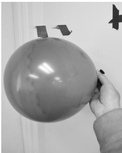
Balloon Rocket. Attach the balloon to the half-straw piece on the fishing line with two pieces of painter's tape. Pinch the balloon neck shut until you're ready to let the balloon rocket fly along the fishing line.
