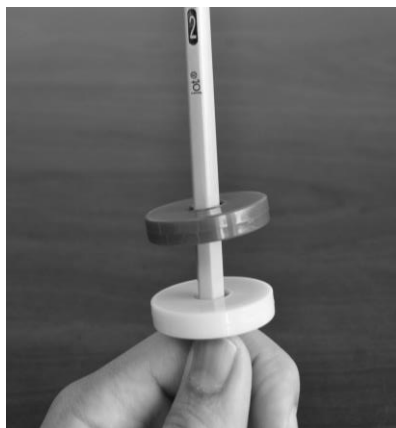
Floating on Air. Stack two ring magnets on a pencil so one floats above the other.
