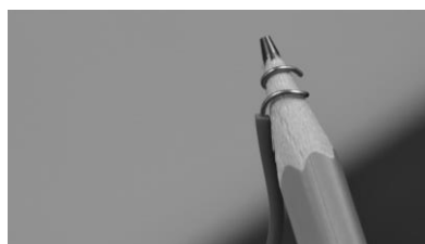
Circuit Flashlight. Wrap one end of the wire around a pencil tip to make a small coil
