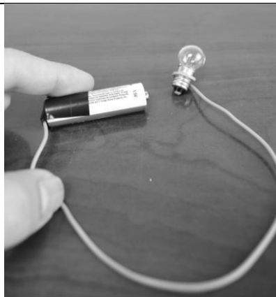
Circuit Flashlight. One end of the wire is taped to the flat (-) end of the battery, and the other end is wrapped around the grooves at the base of the light bulb. You're ready to complete the circuit!
