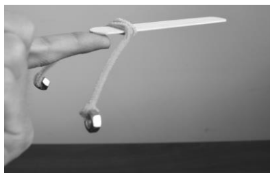
Tightrope Balancer. Create a "Y" shape with the stick and the popsicle stick "arms" so that one end of the Tightrope Balancer perches on a fingertip. (The "arms" will naturally dip below the stick.)
