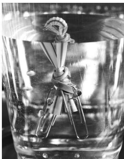
Cartesian Diver. Add paper clips to the rubber band until the top of the diver barely floats above the surface of the water in the cup.
