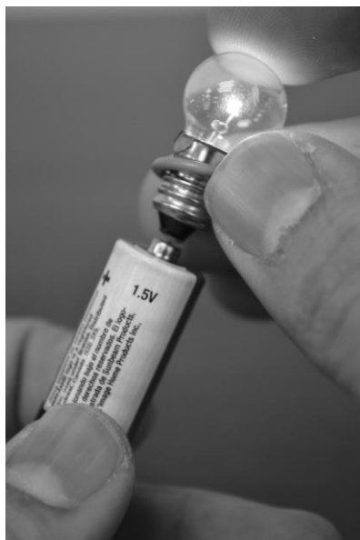
Circuit Flashlight. Holding the wire securely around the base of the light bulb, touch the bottom of the bulb to the (+) nub of the battery.
