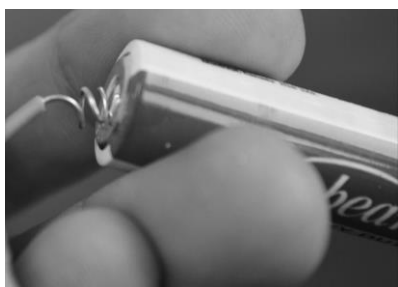
Circuit Flashlight. Wrap one end of the wire around a pencil tip to make a small coil
