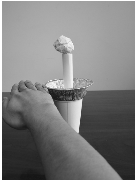
6) Act. 4, Pie Pan & Tablecloth Trick: Set up tower according to curriculum diagram. Chop the small aluminum pie pan sideways so that the paper ball falls into the cup.
