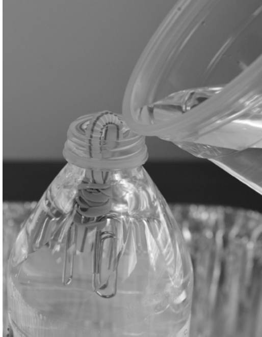
5) Act. 3, Cartesian Diver: Pour water from the 20oz cup to top off the water in the bottle. (The diver is inside the bottle, and the bottle is sitting in the roasting pan to avoid a mess.)
