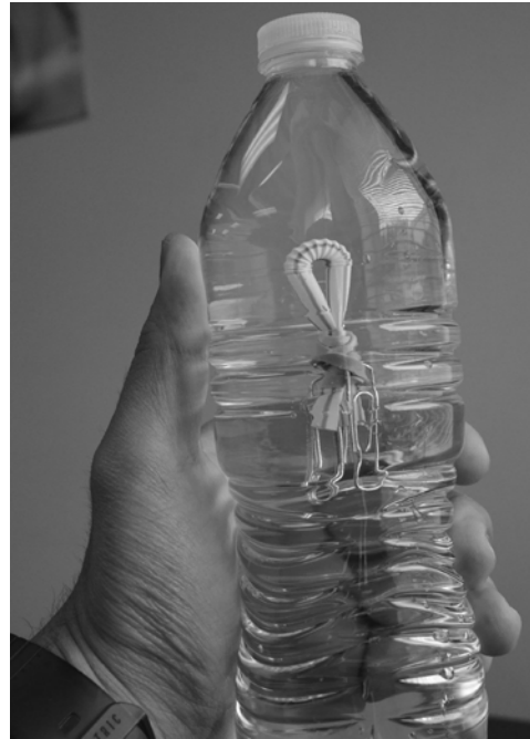
6) Act. 3, Cartesian Diver: When the bottle is squeezed, the diver should sink to the bottom. The diver should float back to the top when the sides of the bottle are released.
