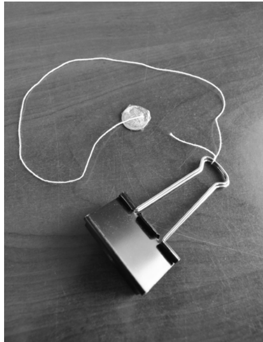
6) Act. 5, Pendulum Drop: Tape the penny to one end of the string and tie the other end of the string to the metal parts of the binder clip.
