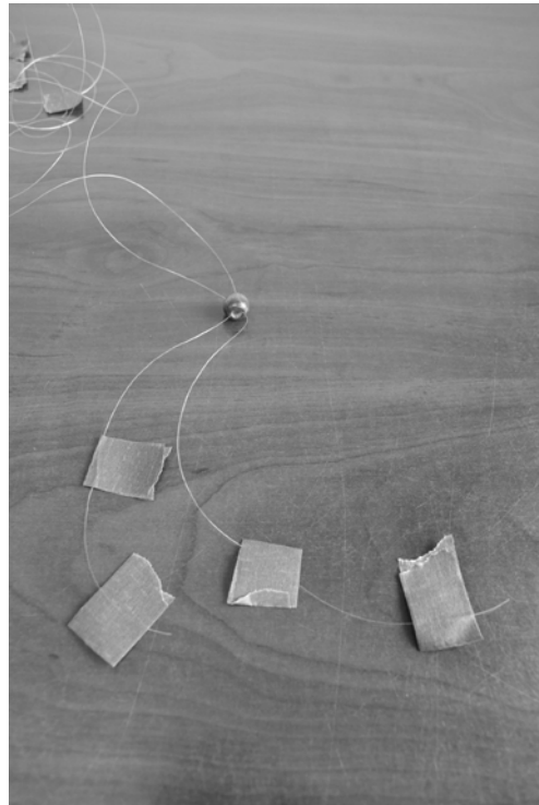
8) Act. 4, Zoom Bead: Thread both pieces of fishing line through the center of the wooden bead. Fold a piece of tape on each of the four ends of the fishing line.
