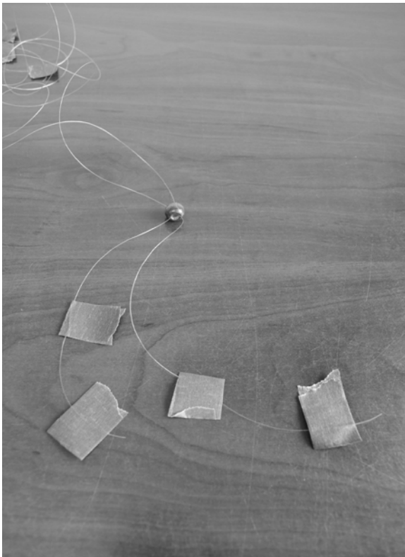
7) Act. 5, Zoom Bead: Thread both pieces of fishing line through the center of the wooden bead. Fold a piece of tape on each of the four ends of the fishing line.
