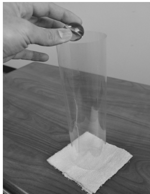
2) Act. 3, Balls, Bounce, & Billiards: The “test chamber” stands upright, with one opening on a folded piece of terry cloth. Drop each ball from the top.
