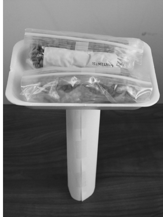
2) Act. 3, Paper Columns: Place the Styrofoam tray on top of a paper column. Attempt to place a pebble bag weight in the center of the tray. If the column can support one bag, it may work best to add a second bag perpendicular to the first one (instead of next to it, as shown).
