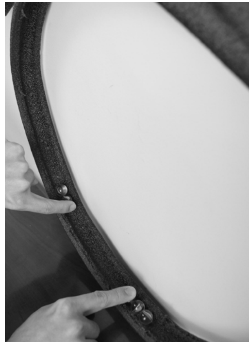
6) Act. 3, Newton's Cradle: While one student holds the center marble still, have another release marbles from above on one side of the track so that they hit the center marble.
