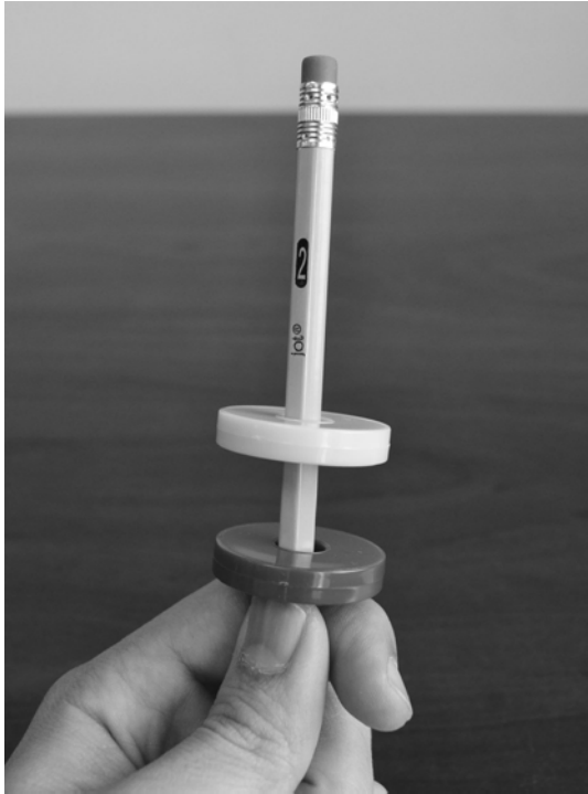
1) Act. 2, Floating on Air: Stack two ring magnets on a pencil so one floats above the other.
