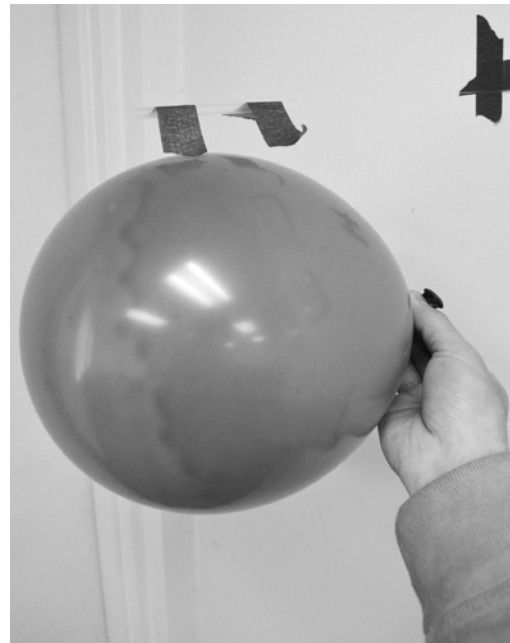
4) Act. 4, Balloon Rocket: Attach the balloon to the half-straw piece on the fishing line with two pieces of painter's tape. Pinch the balloon neck shut until ready to let the balloon rocket fly along the fishing line.
