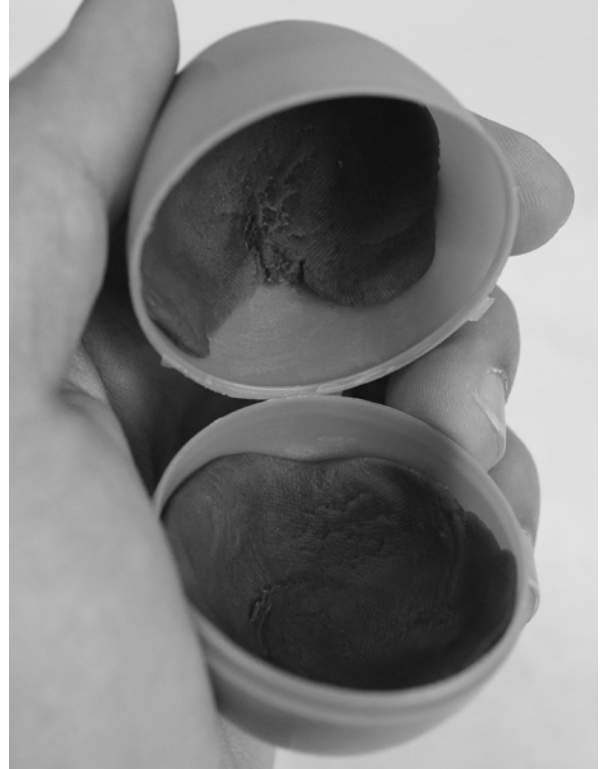
12) Act. 5, Egg Roll: Example of an engineered egg that can roll down the ramp. Note: the play dough is distributed evenly. Roll the egg down the ramp.
