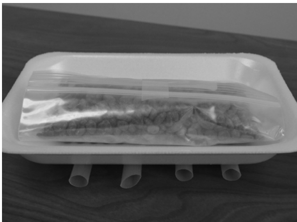
3) Act. 3, What's Friction?: Place the tray on a bed of small wooden dowels (pictured here as straw pieces). The tray should roll over the dowels when pushed.
